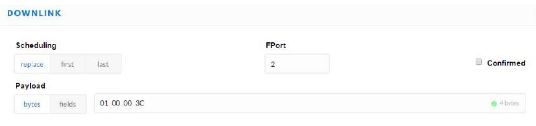
The screenshot shows the TTN Downlink configuration interface. It includes sections for Scheduling (with options for replace, first, and last), FPort (set to 2), and Confirmed (checkbox checked). Under Payload, it shows bytes 01 00 00 3C, which is highlighted in green with a note indicating 4 bytes.
