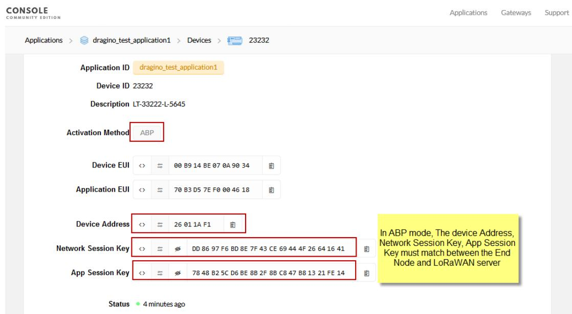
The screenshot shows the DRAGINO Console interface for creating an ABP device. The 'Activation Method' is set to 'ABP'. The 'Device Address' field contains '26 01 1A F1'. The 'Network Session Key' and 'App Session Key' fields are highlighted with a yellow box containing the note: 'In ABP mode, The device Address, Network Session Key, App Session Key must match between the End Node and LoRaWAN server'.
